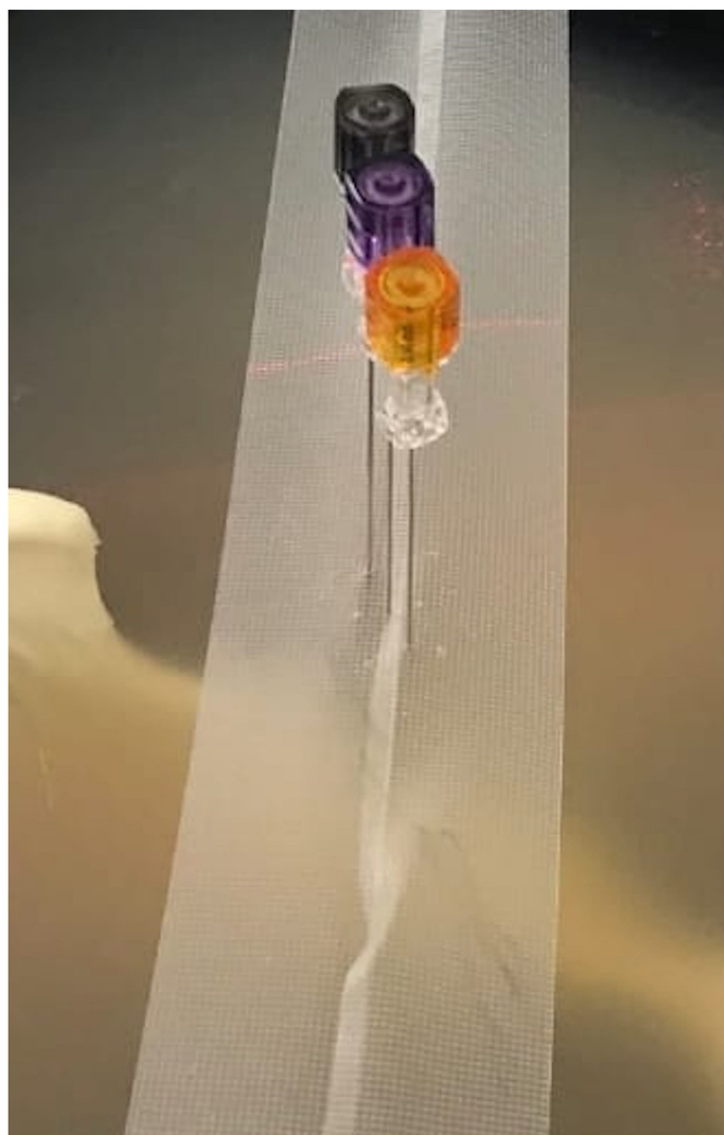
Fig. 1. Total hip arthroplasty phantom. 25, 24 and 22 gauge needles positioned into the phantom at the maximal site of cross section of the metal to give the greatest degree of prosthesis related artefact.
